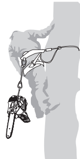
Fig. 37: Example of attachment of tree service chain-saw to centre rear midpoint on harness
