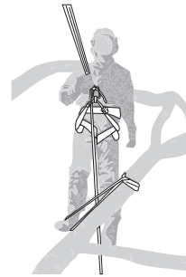
Fig. 39: Example of temporary foot stirrup created from endless sling
